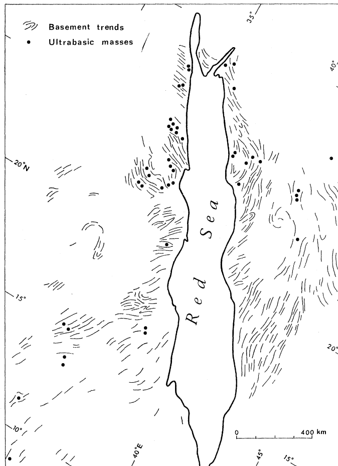
FIGURE 13. Compilation of basement trend lines and ultramafic occurrences adjacent to the Red Sea.
